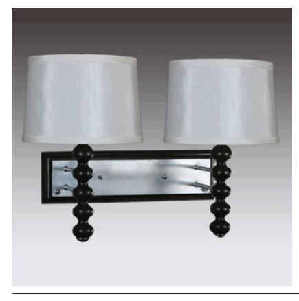
16" Expresso/Brushed Nickel Double Wall Lamp, two medium base sockets, two on/off push button switches at backplate, 8' Silver 45°cord, 24" matching cord cover. Includes (2) 8.5"x9.5"x7" Winter White Hardback Shade, recommend two 1100 lumen LED bulbs.
